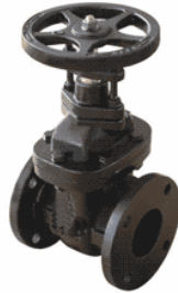
FIG. 275-CI-125 Class 125, Flanged ends, bolted bonnet, Cast Iron body & bonnet, Bronze trim.
