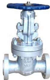
FIG. 272-CS-600 Class 600, Flanged ends, bolted bonnet, WCB body & bonnet, 13Cr/HF trim.
