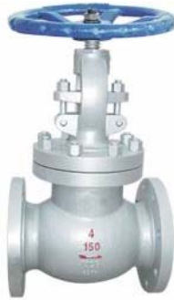
FIG. 276-CS-150 Class 150, Flanged ends, bolted bonnet, WCB body & bonnet, 13Cr/HF trim.
