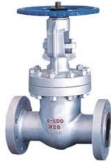
FIG. 276-CS-600 Class 600, Flanged ends, bolted bonnet, WCB body & bonnet, 13Cr/HF trim.
