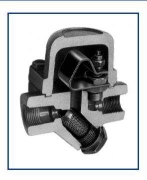
Designed for fast start-up and modulating discharge with no live steam loss on services up to 30 psig. Ideal where a forged body with "Y" type strainer is required to handle light condensate loads including low pressure dripleg.
