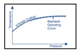
Following the steam curve is the key to efficient steam trap performance. Utilizing dual thermostatic/thermodynamic forces allows Bestobell delta traps to match the steam curve, meaning that the energy in the steam is efficiently used by the process and not wasted in operating the trap.
