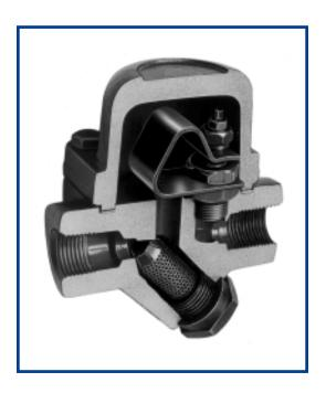
The DM25 is a high performance, energy efficient steam trap that incorporates a Y-type strainer and integral check valve. For use on steam main dripleg and critical tracing service with differential pressures to 320 psig.
