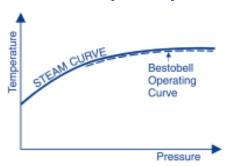
Following the steam curve is the key to efficient steam trap performance. Utilizing dual thermostatic/thermodynamic forces allows Bestobell delta traps to match the steam curve, meaning that the energy in the steam is efficiently used by the process and not wasted in operating the trap.
