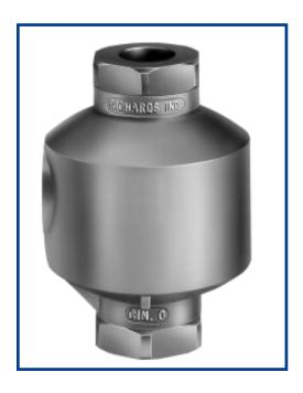
A lightweight steam trap for plant applications requiring sealed stainless steel construction. Easy to install for steam main dripleg and critical tracing services with differential pressures up to 150 psi (10.34 bar).
