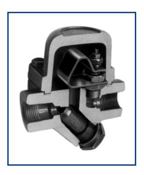
A series of compact, high capacity steam traps developed to handle the varying loads and pressures typical of process and heating applications with differential pressures to 320 psi. Featuring a built-in strainer and check valve, the M25/GM25 is produced in sizes up to 2".
