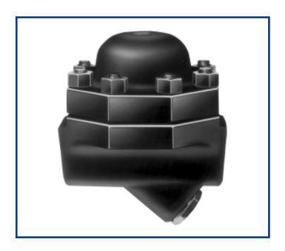
A series of heavy-duty steam traps in 1-1/2" & 2" sizes designed specifically for high pressure, high flow process applications. Featuring built-in Y-type strainers and check valves, this series can be used for services with differential pressures up to 900 psi (62 bar).
