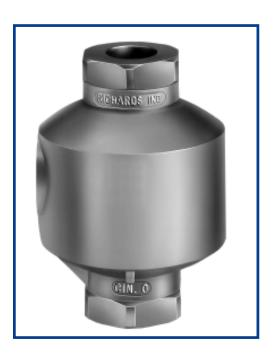
Bestobell's TS22 is a lightweight trap designed for applications requiring sealed stainless steel construction. For services with up to 300 psi differential pressure, this model is designed to efficiently make use of the sensible heat by retaining condensate within the tracer line.
